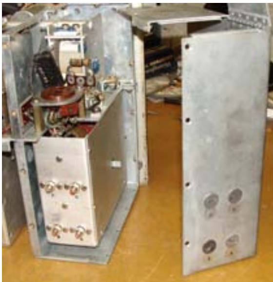
What is essentially the entire right side of the radio (as viewed from the rear) had to be removed to gain access to the r.f. oscillator compartment.
