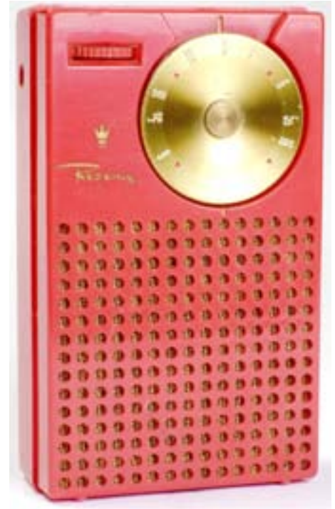
Regency TR-1 – the world's first transistor radio (circa 1954/55) was made in the U.S. and used a 4 (germanium) transistor circuit.
