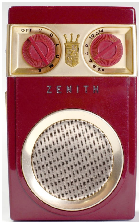
Zenith's first transistor radio, the Royal 500 (circa 1955), featured a hand-wired chassis, made in the U.S. and using a 7 transistor circuit.
