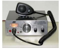
The control panel is simplicity itself. A tuning knob adjusts the frequency (28.3-28.6 MHz), and a volume control selects comfortable audio from the internal 3" speaker.
