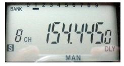
Memorization is done in the conventional manner: Choose a vacant channel, or an assigned channel that you want to overwrite, and press the program key (PRG) followed by the frequency; then press PRG again.
