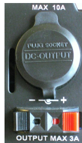
Power is available on the front panel cigarette lighter jack and push terminals
