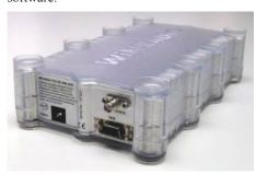
There are many advantages to this approach, especially the flexibility of demodulation modes - new modes can be added easily by simply upgrading software. The G33EM also performs better than a comparable conventional receiver, thanks to advanced signal processing techniques which make it possible to implement sharper selectivity filters, and more accurate demodulators and decoders than conventional hardware.
